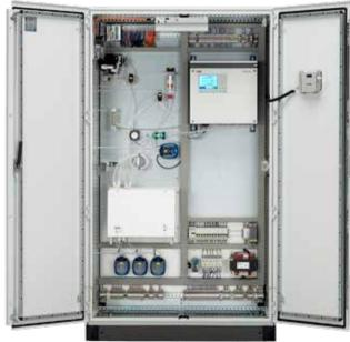
An extractive analysis system for general and specialised use. The system can be configured with two 19" analysis modules. A controller and operator interface can be installed on this system. The system is available with a variety of communication options
